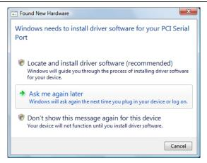
Click on Locate and install driver software (recommended). Windows will guide you through the process of installing driver software for your device.
